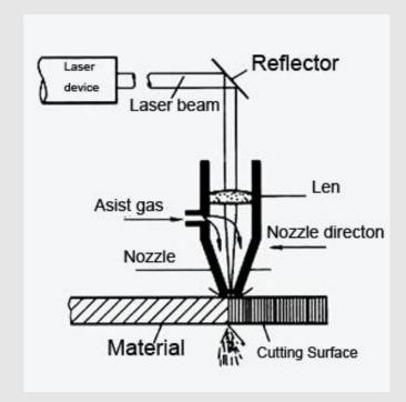
Compressed air with fog and oil will affect the beam transmission and lead to seriously focus decentralization when spray to lens, finally result in incomplete piercing and defect products.
